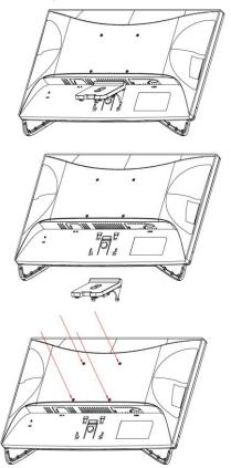
This monitor can be attached to a wall mounting arm which can be purchased separately. Disconnect power before this procedure. Follow these steps:
